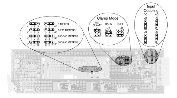
Figure 8-7. VPD-6830-XEQ Jumper Locations
